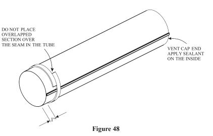
**Note:** Tape gasket to be applied prior to installing to fireplace flue outlet tube only. Tape gasket should not be used when mating the flue outlet tube to a rigid venting system.
